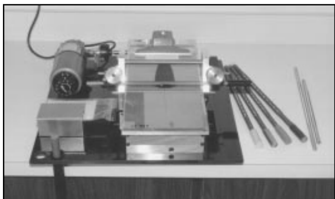
Figure 2. Automated draw down system using wire wound metering bars.
