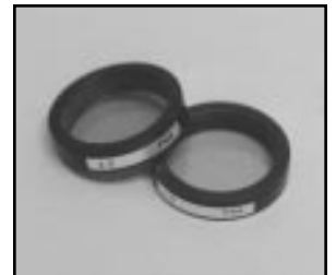
Figure 18. Tensioned ring gauges.
