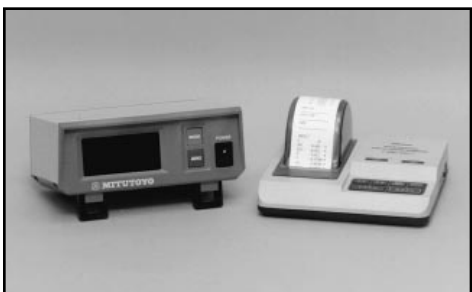
Figure 14. A statistical processing printer and electronic read outs provide quick process information for statistical process control (SPC.)
